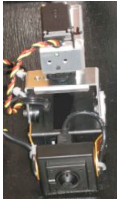
2-Axis (Pan & Tilt) Camera gimbal with options for roll axis & active stabilization.
